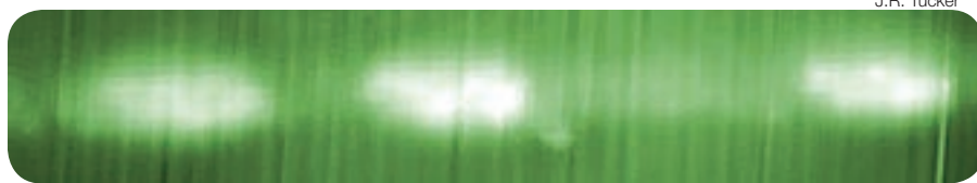
Cross-section scanning tunneling microscope image shows InAs quantum dots—about 30 nm long—embedded in gallium arsenide.
