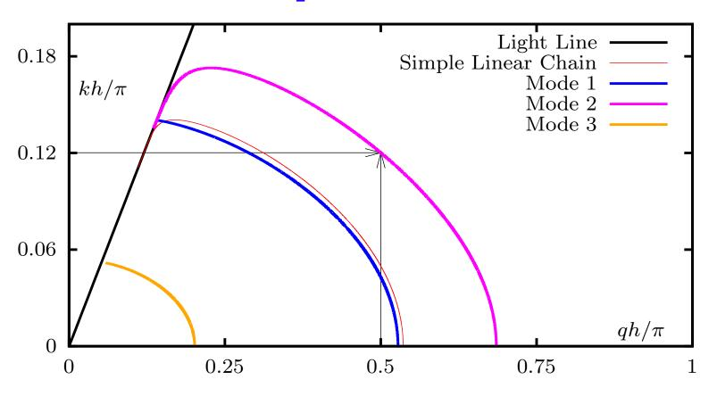
Simulation for prolate spheroids; h=25.3nm, H=2h=50.6nm, a=6.325nm, b=42.17nm Drude metal with eps\_0=5.0
